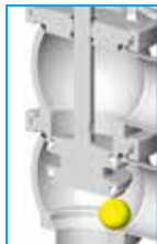
DCX4 particle passage closed valve
