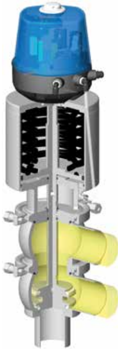
CLOSED POSITION Upper line flow
