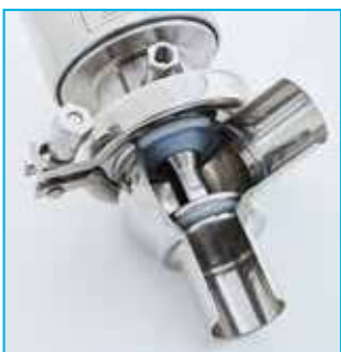
DCX3 diaphragm valve fitted with a stainless steel plug with a floating PFA seal and a PTFE deformable diaphragm
